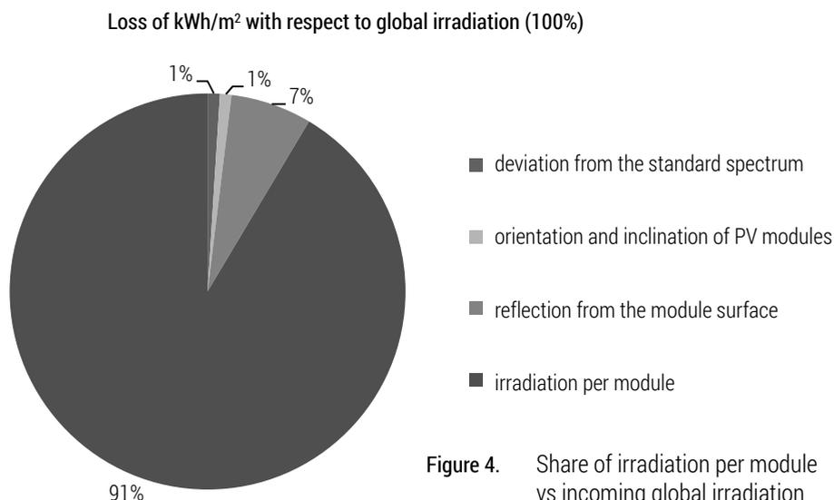
**Figure 4.** Share of irradiation per module vs incoming global irradiation
