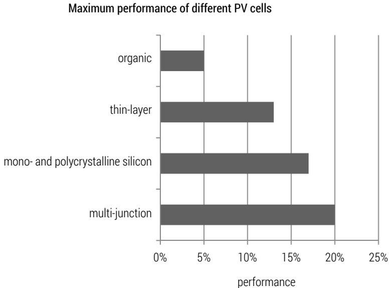
**Figure 2.** Performance of different types of PV cells
