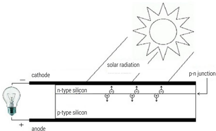
**Figure 1.** Schematic representation of a photovoltaic cell
