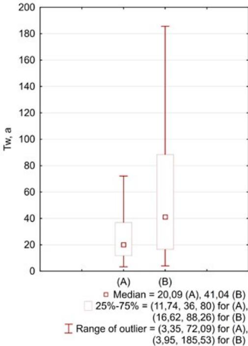
Figure 7. Summary of risk calculations for the water networks (A) and (B): the average working time without failures –  $T_w$
