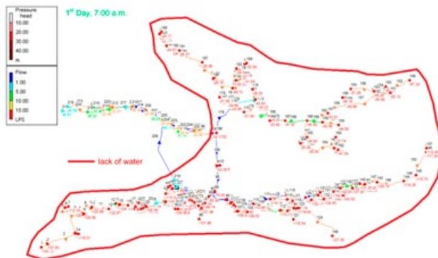
Figure 4. Simulated failure of water pipe section no 226 – the first to the third hour of failure-free operation – no 226
