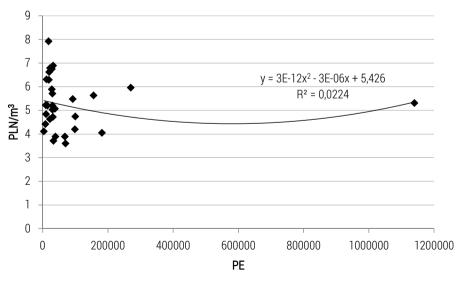
**Figure 4**. Prices for treatment of domestic sewage in treatment plants with increased nutrient removal depending on the designed p.e.
