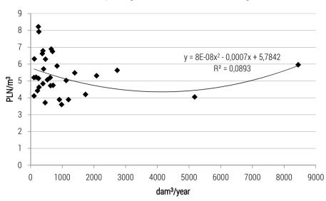
**Figure 3**. Prices for treatment of domestic sewage in treatment plants with increased nutrient removal depending on the amount of treated sewage
