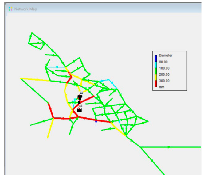
Figure 8. Diameters of water supply network pipes
