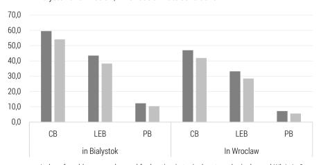
■ Index of usable energy demand for heating in typical meteorological year, kWh/a/m2
