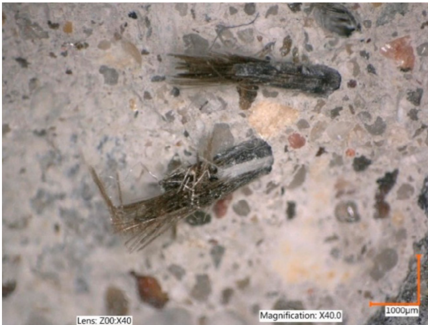
Figure 3. View of the cracked cross-section after failure
