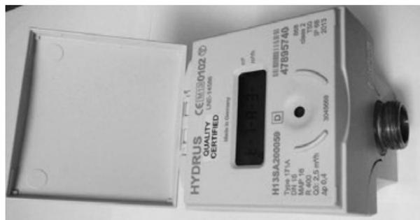
**Figure 3.** Electronic static water meter
