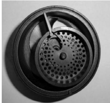
**Figure 2.** Rotor of a volumetric flow meter
