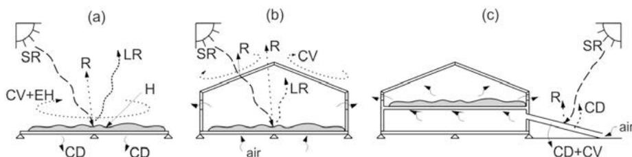
**Figure 3.** Working principles of (a) open sun drying, (b) direct sun drying and (c) indirect solar drying: CD – conductive losses, CV – convective losses, EH – evaporative heat losses, H – heat absorbed, L – low wavelength radiation, R – radiation, SR – short wavelength solar radiation
