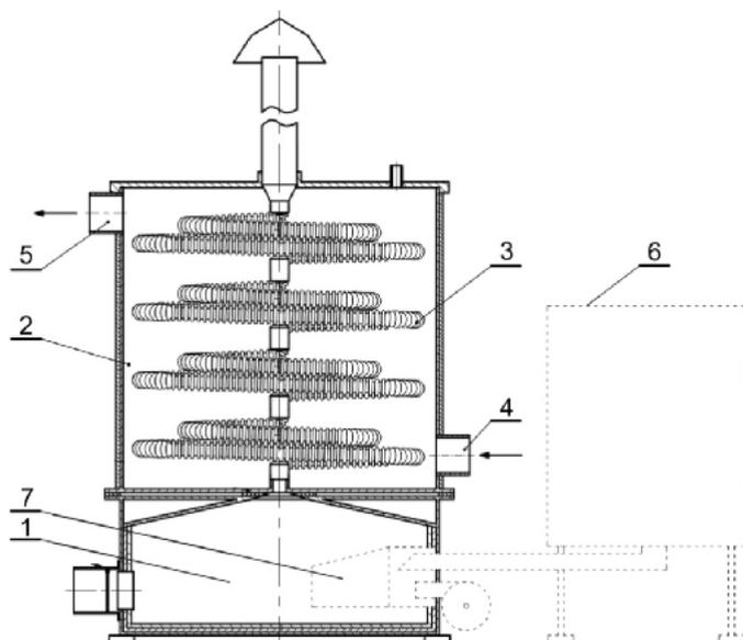
**Figure 7.** The air heater equipped with biomass stove: 1 – combustion chamber, 2 – heat exchanger, 3 – tubular section of flue, 4 – air inlet, 5 – air outlet, 6 – biomass heating unit with biomass-storage cell, 7 – burner
