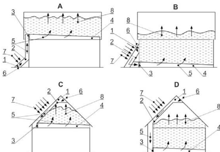
**Figure 4.** Basic rules for installing solar collectors in farm buildings; A – wall collector with drying room in the loft, B – wall collector with dryer in the barn, C – under floor collector with drying room in the loft, D – under roof collector with drying room in the barn; 1 – air inlet, 2 – collector, 3 – fan, 4 – distribution channel, 5 – heated air, 6 – ambient air, 7 – solar radiation, 8 – humid air
