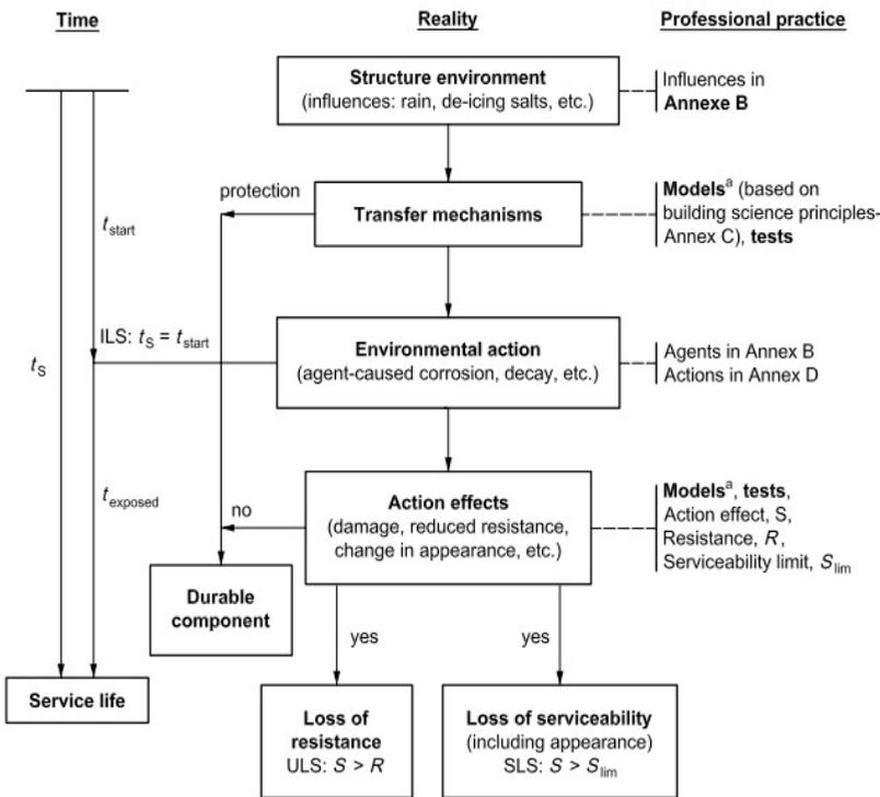
Figure 2. Design durability limit state
